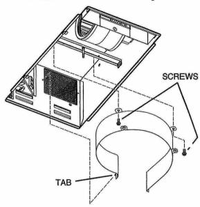
Install new scroll band into housing. Insert <u>tab</u> on scroll band into hole in housing and secure with two (2) <u>screws</u> provided.
