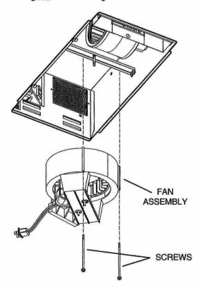
Unplug motor and remove two (2) screws holding <u>fan</u>
