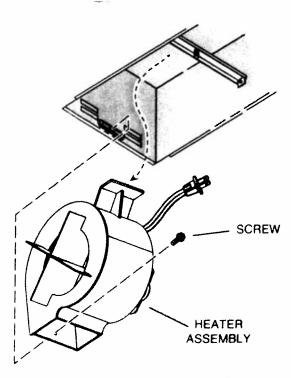
Unplug motor and remove screw holding heater assembly in place. Remove heater assembly from housing.
